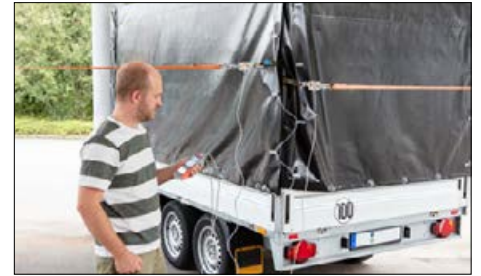
Measurement of forces in different tensile or compression directions possible with only one measuring device
