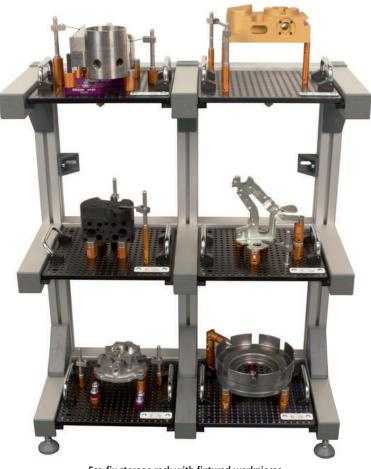
Eco-fix storage rack with fixtured workpieces
