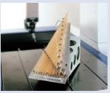
CMM calibration using a virtually zero thermal expansion glass gauge
