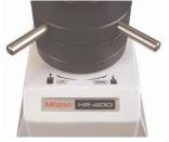
handle auto start feature. Motor drive controls loading
