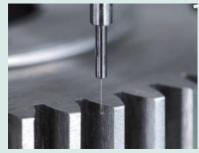
MPP-NANO Module 0.8 master gear measurement
