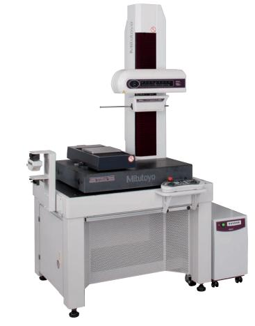
SV-C4500CNC equipped with two powerful exchangeable drive units
