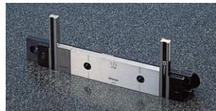
Holder B and C: Used for coupling two long gauge blocks together with other gauge blocks up to 35 mm (Holder B) or 140 mm Holder C). Also used for attaching jaws with two adapters. Holder B : 619032 (R max.= 90 mm- L= 126 mm) Holder C : 619033 (R max.= 200 mm- L= 236 mm)
