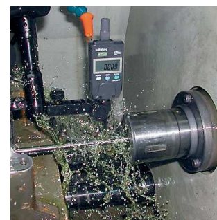
Rated to IP66 water-and dust-proofing standard, and oil resistance improved.
