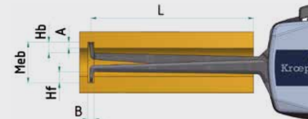
Meb Measuring range Hb Measuring contact movable A Groove depth Hf Measuring contact fixed B Groove width L Measuring depth
