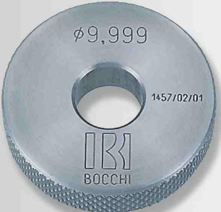
**Ring gauges** in a special steel-chrome alloy 90MnVCr8KU. Excellent resistance to wear, core-hardened hardness >62 HRC, tempered and stabilized. Rings with measurement etched and suitable for calibration of comparison instruments are available upon requirement.
