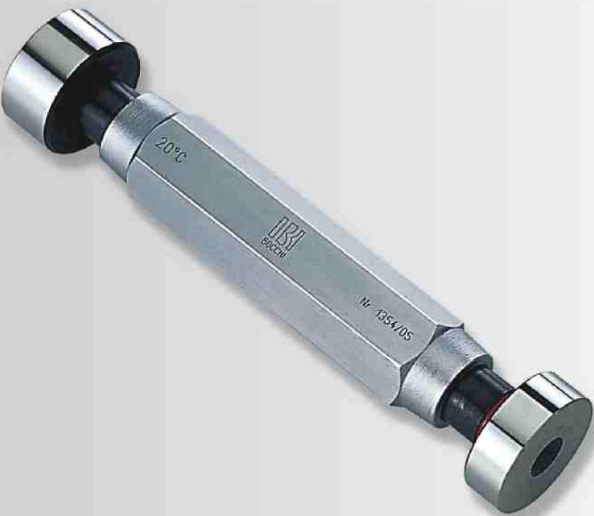
**Cylindrical plug gauges "Go-No Go"** in a steel-chrome alloy 90MnVCr8KU. Excellent resistance to wear, core-hardened hardness >62 HRC, tempered and stabilized. Available from Ø 3 to Ø 100 mm to tolerance H7. Can be supplied in different tolerance classifications upon requirement.
