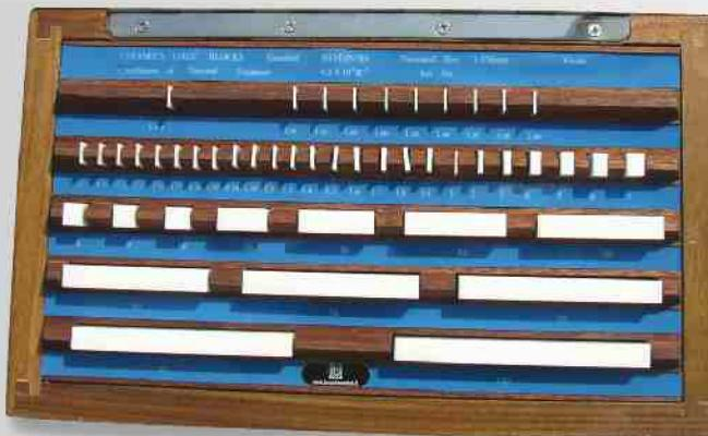
**Set of exceptionally pure ceramic zircon parallel gauge blocks.** The physical and mechanical properties of ceramic zircon offer the following advantages: an expansion coefficient similar to the steel; high thermal stability; high resistance to abrasion and wear; resistance to corrosion; good cohesion capacity; mechanical resistance with values similar to steel. Serial number on each block. Manufactured as per UNI EN ISO 3650. Supplied in case. Available at grade 0 and 1.
