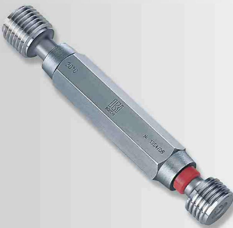
**Thread plug gauges** in high wear-resistant steel-chrome alloy. Core-hardened, tempered and stabilised. Normally constructed gauges for the following thread types: Metric, Withworth, Cylindrical gas, Tape gas, Acme, American unified UNC, UNF, UNEF. The thread plug gauge is supplied to tolerance 6H in the standard versions.
