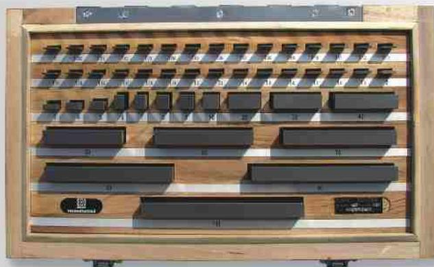
**Set of tungsten carbide parallel gauge blocks.** Tungsten carbide has the following advantages over steel: a much lower expansion coefficient with greater stability even at temperatures other than the reference; greater hardness (1500 Hv) and therefore more long-lasting; it does not require protection from oxidation; perfect adherence. Serial number on each block. Manufactured as per UNI EN ISO 3650. Supplied in case. Available at grade 0 and 1.
