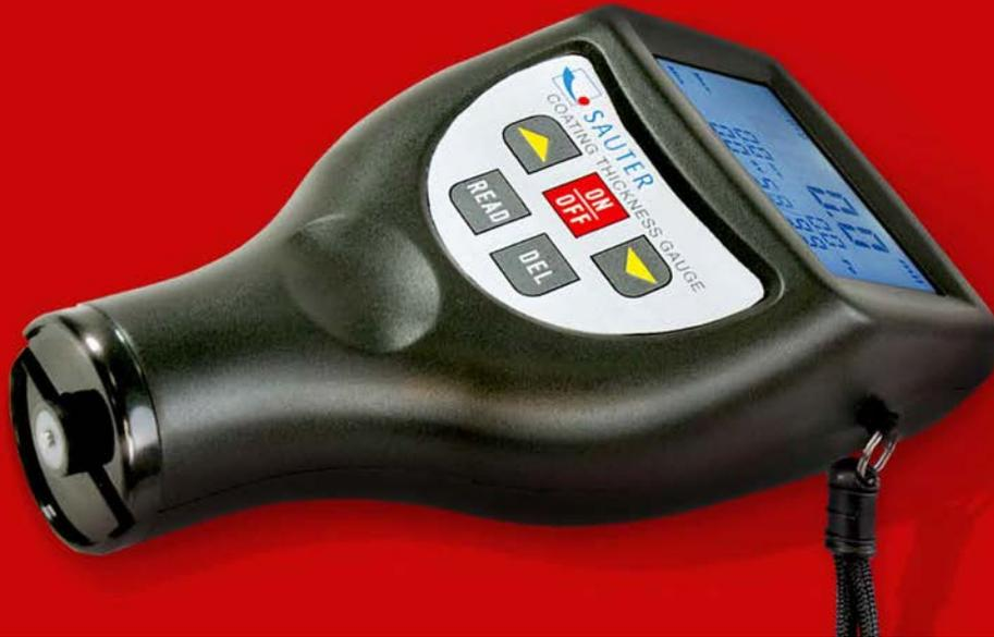
Measurement of coating thicknesses is known from, for example, the paint measurement for coating thickness at cars. In fact, these measurements are used much more widely in industrial applications. This is where the thickness of the surface finish is measured, such as galvanisation, zinc coating etc, or also lacquers.
