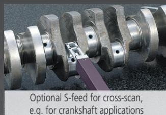
Optional S-feed for cross-scan, e.g. for crankshaft applications
